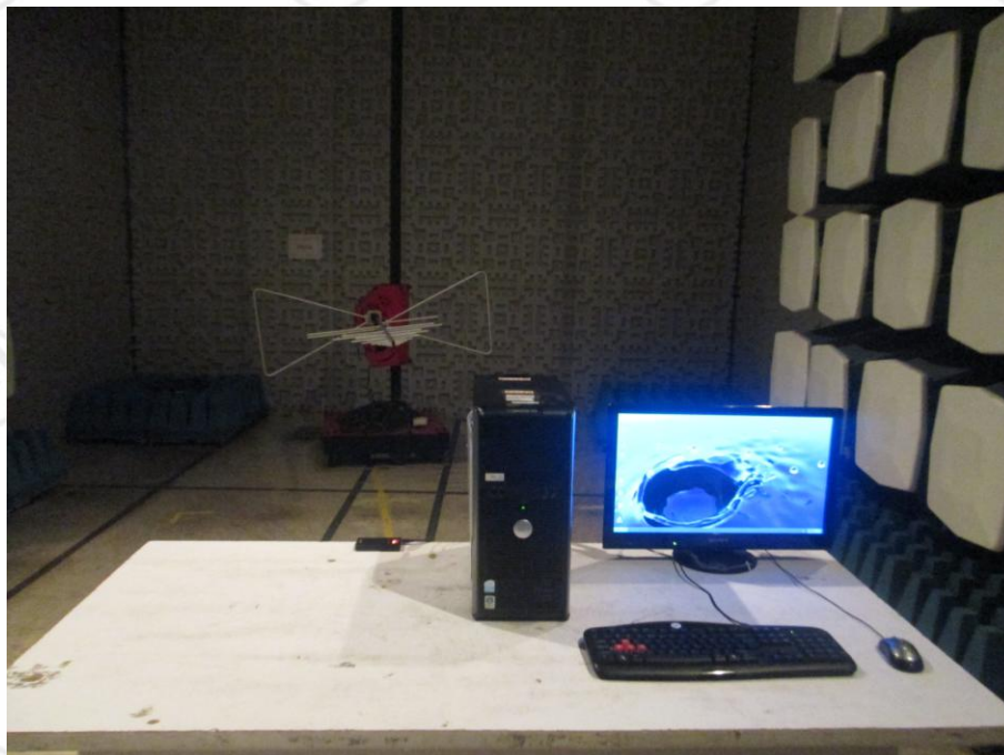
RADIATED EMISSION TEST SETUP (CHARGING)
