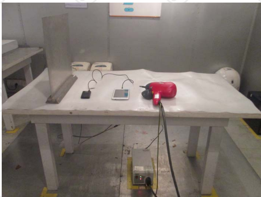
ELECTROSTATIC DISCHARGE TEST SETUP (DISCHARGING)
