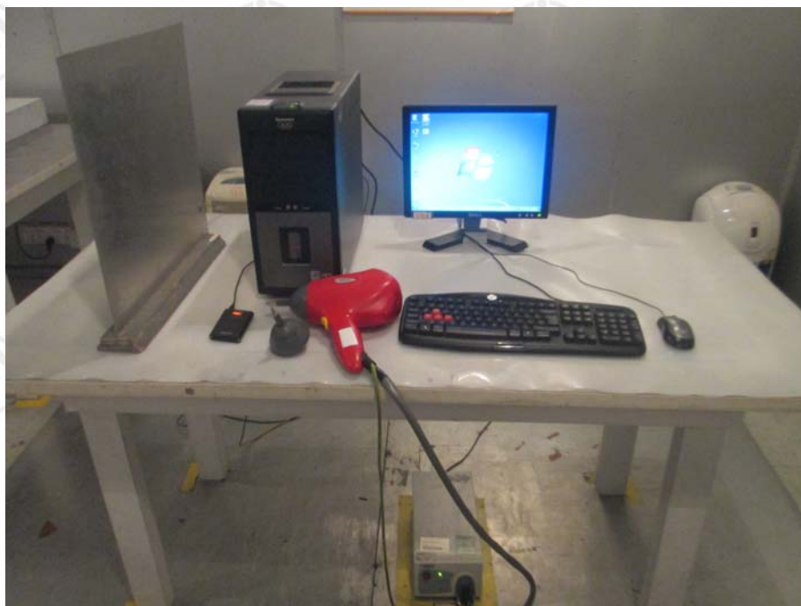
ELECTROSTATIC DISCHARGE TEST SETUP (CHARGING)
