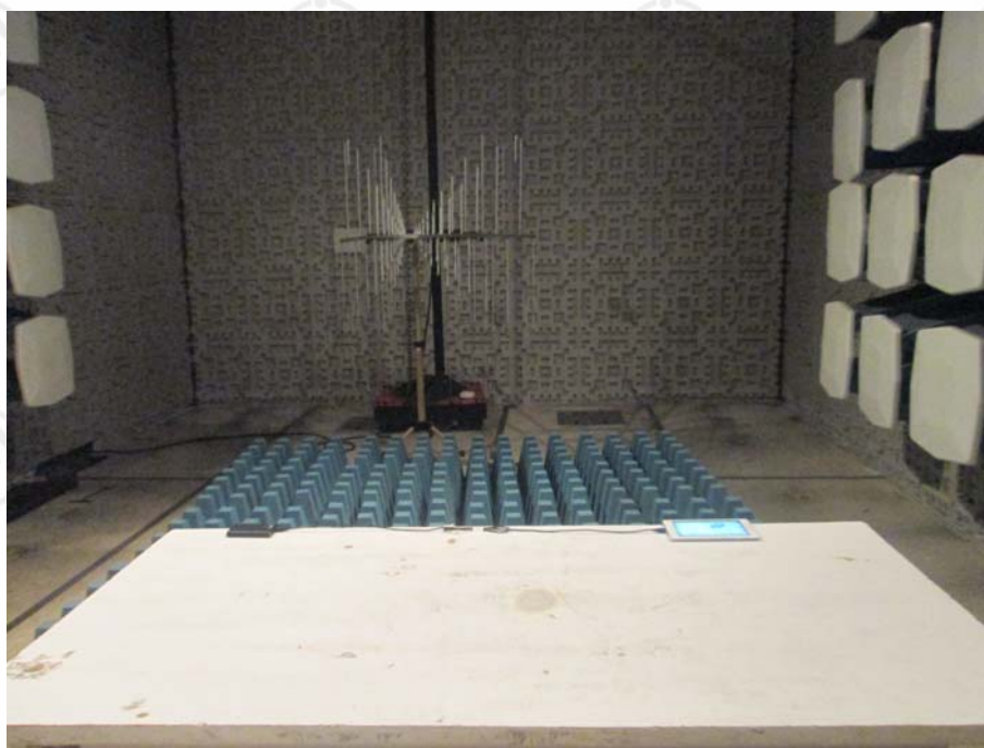
RADIO-FREQUENCY ELECTROMAGNETIC FIELD TEST SETUP (DISCHARGING)
